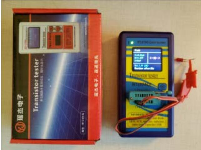
little device has an internal processor and a color screen and a variety of ways to connect 2 and 3 terminal devices including resistors, capacitors, inductors, diodes, LEDs, and transistors. It figures out what the device is, what lead is connected to what input, and displays the readings relative to the device under test along with a graphical picture!
