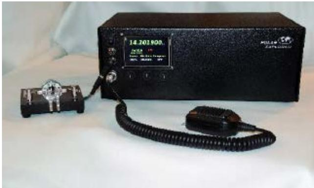
**Polar Explorer** is a 500 watt transmitter, only, but offering significant efficiency on the order of 88% as opposed to a typical value of under 60% in SSB service. The owner was soliciting beta testers who would agree to buy the hardware, at parts cost, and help with further development. The rig was designed to use another rig as a receiver, such as an Elecraft K2, at a cost less than an external linear amplifier. More could be seen at <https://www.polex-tech.com/>
