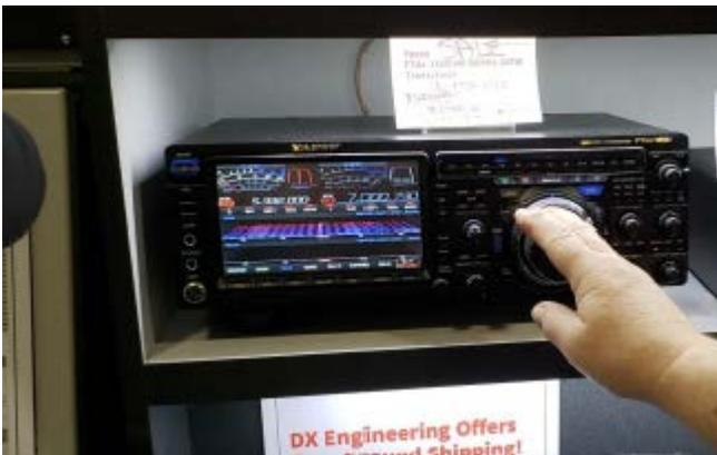
**Yaesu** had examples of the new FT101D radio at several locations, including DX Engineering. This under \$4000 rig (100W version, the 101MP is a 200W radio) had a unique 3-D waterfall that provided both signal strength and waterfall history on the display, and could separate the waterfall between the main and sub receivers.
