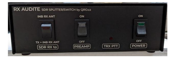
In my ham shack I have several SDR receivers that I like to use along with my main transceiver. I have only one antenna for 0.1 to 30 mHz so it is a benefit to seamlessly share this antenna with my SDR receivers and my transceivers. The RX Audite does exactly that. It provides antenna sharing with the SDR receivers while offering them protection from excessive RF coming from my transceivers.
