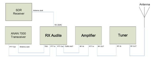
Here is a simplified diagram of how the RX Audite is connected to my equipment. The RX Audite is connected between the transceiver and amplifier. The Audite is only exposed to the lower RF power from the transceiver and not the high RF power from the amplifier. Muliple SDR receivers can be connected to the RX (SDR) port using an RF power splitter.
