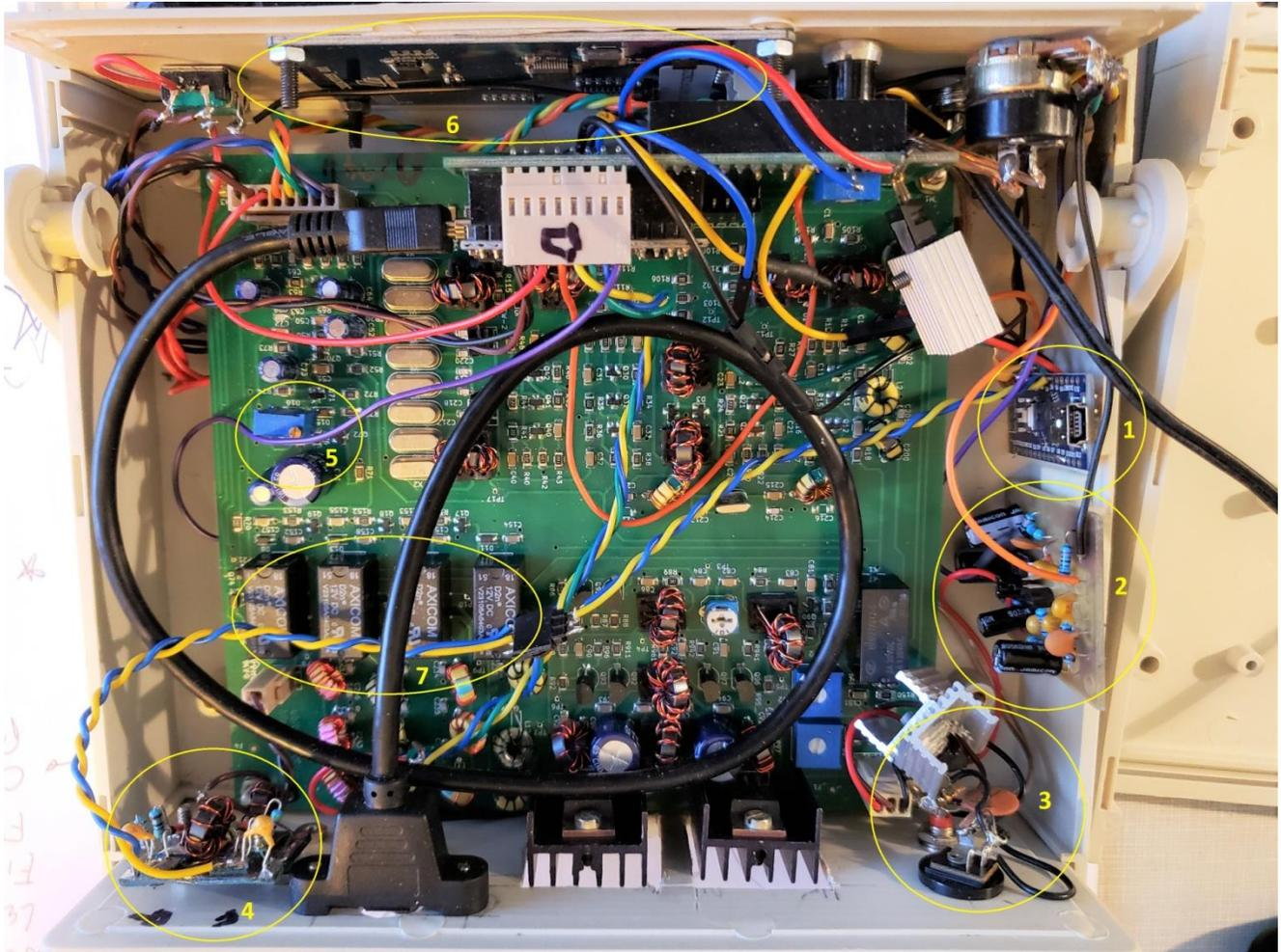
1. This is an outboard Arduino Nano board that links to the main Raduino board and adds several features including: A DSP S-Meter (replacing a simple audio amp circuit), a CW decoder, SWR logic, and an audio spectrum display. This (like the incorporation of the touch screen) comes from the mind of KD8CEC and you can see it at <http://www.hamskey.com/2018/07/standalone-signal-analyzer-i2c-type.html#more>
